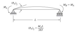
COMPATIBILITY  $\theta_A = (\theta_A)_1 - (\theta_A)_2 = 0$ Substitute for  $(\theta_A)_1$  and  $(\theta_A)_2$  and solve for  $M_A$ :  $M_A = M_B = \frac{5q_0L^2}{96}$  **Problem 10.4-6** A continuous beam *ABC* with two unequal spans, one of length L and one of length 2L, supports a uniform load of intensity q (see figure).
