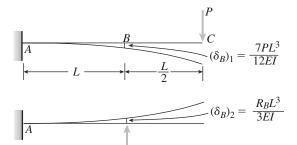
COMPATIBILITY  $\delta_B = (\delta_B)_1 - (\delta_B)_2 = \frac{R_B}{k}$ Beam *DE*:  $k = \frac{48 EI}{r^3}$
